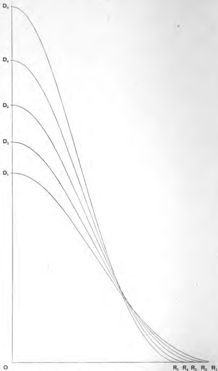
D_1 R_1, D_2 R_2, D_3 R_3, D_4 R_4, D_5 R_5 , are density curves, corresponding respectively to the temperature curves T_1 R_1, T_2 R_2, T_3 R_3, T_4 R_4, T_5 R_5 , of figure 1.
